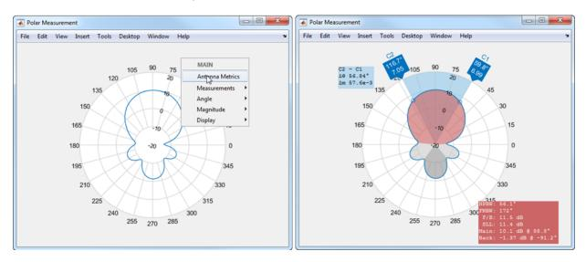
By default, the plot shows the HPBW (half-power beamwidth) of the antenna. The antenna measurements text box displays:
